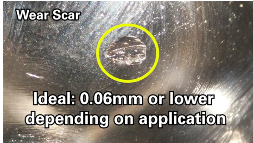
Figure 1: A ball wear test shows the wear scar measurement on a lubricated surface. A smaller wear scar indicates better protection against metal-to-metal contact. High-performance extreme pressure greases with molybdenum disulfide or other anti-wear additives help extend component life by reducing friction and wear. Courtesy: CITGO Petroleum
