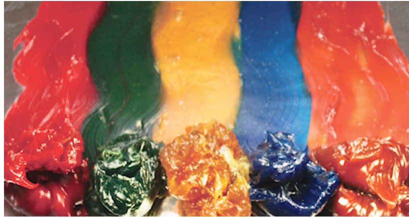
Figure 3: Grease color is often determined by dye additives and does not indicate performance characteristics. The choice of thickener, base oil and additives is what determines grease suitability for different applications. Courtesy: CITGO Petroleum
