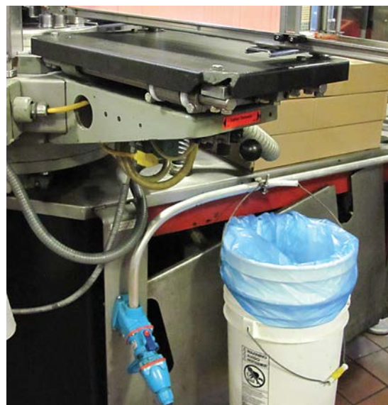
Meltric DECONTACTOR™ Series switch-rated plugs and receptacles can safely make or break electrical loads. They are a NEC-approved 'line of sight' disconnect switch, as shown here on a glass bottle labeling machine.
